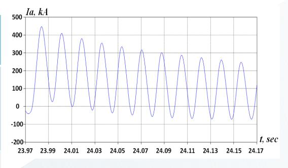
Phase A current with a two-phase s/c passing into a three-phase s/c, lamax = 446,6 kA
