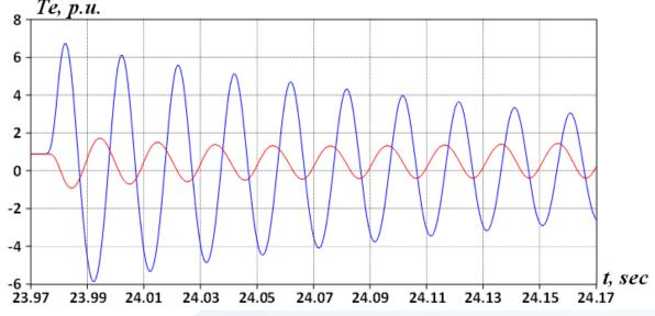
Change of electromagnetic torques created by three-phase systems in idle mode (blue curve - emergency winding, red curve circuit-free winding)
