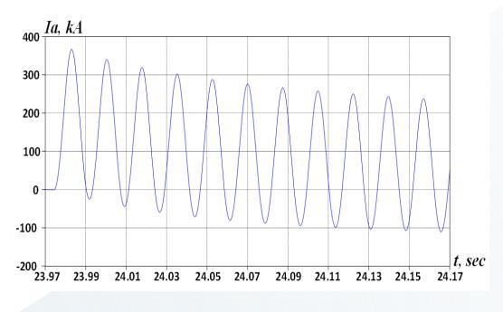
Phase A current at three-phase s/c in idle mode, Iamax = 367,2 kA
