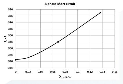
Dependence of the short circuit current amplitude value at three-phase short circuit on the mutual reactance along the leakage paths between three-phase systems (T3V-1200-2A, rated load mode)
