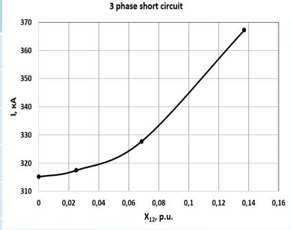
Dependence of the short circuit current amplitude value at threephase short circuit on the mutual reactance along the leakage paths between three-phase systems (T3V-1200-2A, idle mode)
