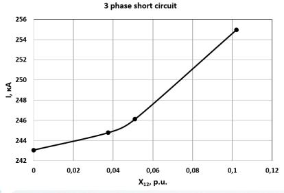
Dependence of the short circuit current amplitude value at three-phase short circuit on the mutual reactance along the leakage paths between three-phase systems (TVV-1200-2, idle mode).
