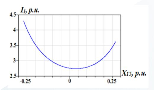
Dependence of the short-circuit current at the terminals in one of the generator windings on the mutual reactance along the leakage paths between three-phase systems
